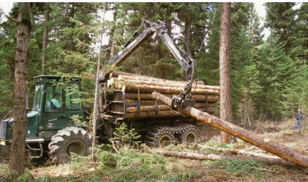
Logger Dale Flannigan operates a low-ground pressure log forwarder in a forest thinning operation near Missoula, Mont. The forwarder gathers and removes felled logs, carries them to a landing for loading on a truck, and allows thinning to be done with a minimum of road building.
