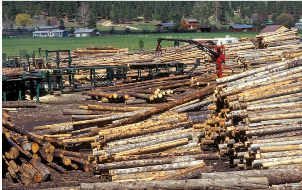
Charred logs from a forest fire are sorted for processing into boards at a sawmill in northern Idaho. Salvage of logs from a fire must proceed quickly since after a fire the trees are attacked by insects and disease and within a matter of months are no longer usable.
